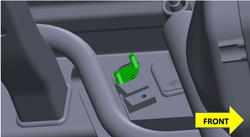
Figure 12- Driver Side Nut Plate Installation
